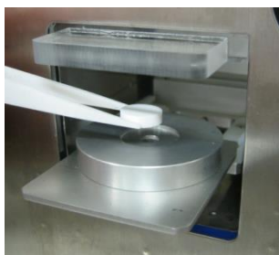
Sample compartment (dry air purged)
